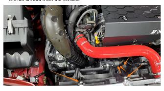
3. Using a 12mm socket, remove the bolt securing the stock charge pipe to the engine. Then, using a flathead screwdriver or pick tool, disengage the spring clip at each end of the stock charge pipe and remove the charge pipe from the vehicle.
