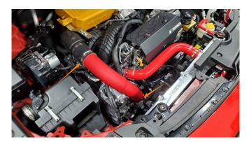
7. Using a 12mm socket, secure the Mishimoto charge pipe to the engine using the supplied washer and the bolt that was removed in Step 3.
