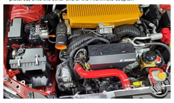
6. Install the lower end of the Mishimoto charge pipe onto the turbo outlet until the spring clip snaps into place. Applying a light coating of clean motor oil to the outside of the turbo outlet and inside of the charge pipe will aid in installation. Install the upper end of the Mishimoto charge pipe into the Mishimoto coupler and secure it with the 70-90mm worm gear clamp. The four
