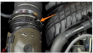
4. Using a flathead screwdriver, loosen the clamp securing the stock coupler to the intercooler pipe and remove the coupler and clamp from the vehicle.
